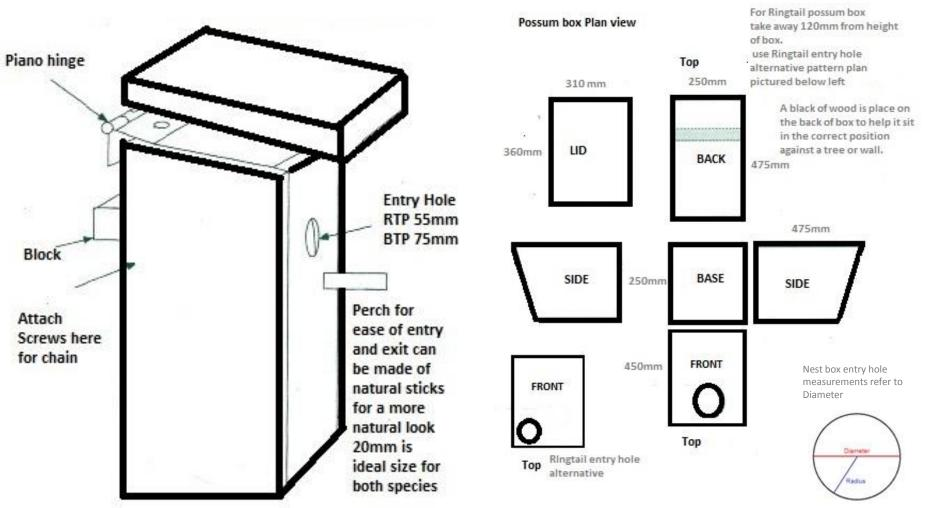
Box should be made from 7-9 mm Marine ply to ensure weather proofing , you can use normal ply but you must paint box with 2-3 coats of acrylic paint to help with weatherproofing drill 1 single 3mm hole in the middle of base to allow water to escape, should it get wet during storm conditions, over hang of lid should prevent rain entry
