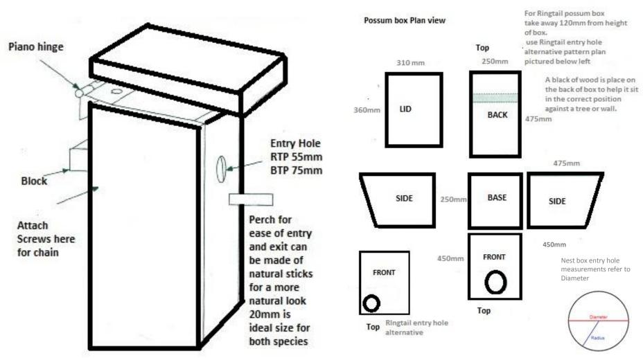
Box should be made from 7-9 mm Marine ply to ensure weather proofing, you can use normal ply but you must paint box with 2-3 coats of acrylic paint to help with weatherproofing. Drill 1 single 3mm hole in the middle of base to allow water to escape, should it get wet during storm conditions, however over hang of lid should prevent rain entry.
